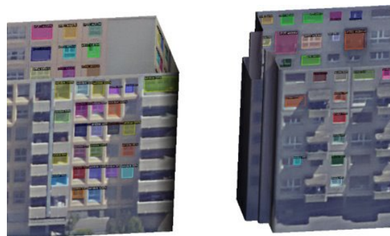
Figure 4. Overview of the window detection performed on the facade ortho-images and reprojected on the 3D model of the buildings of the demonstration area.
