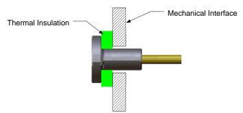
Figure 6. Thermal insulation at mechanical interface
