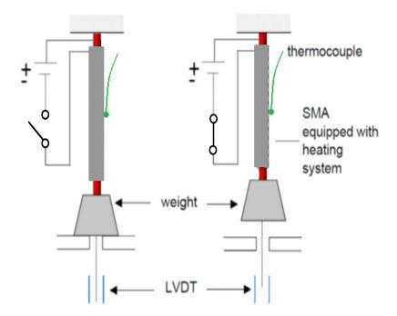
Figure 10. Schematic drawing of the equipped SMA wire test jig
