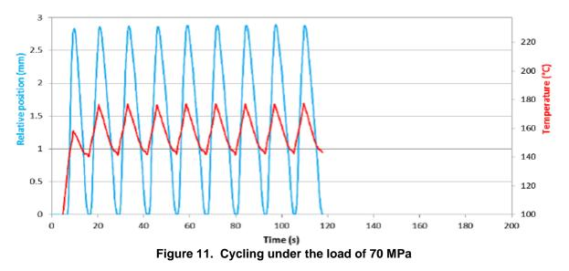
Figure 11 shows a uniform cycling demonstrating the adequate behavior of the wire at 70 MPa. The same test was performed at 40 MPa demonstrating its ability to reset fully at this stress level.
