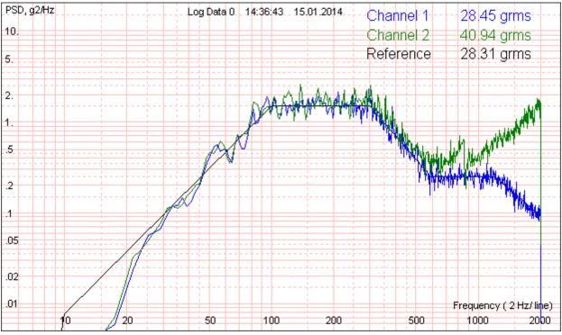
Figure 18. Random vibration spectrum in the axial direction
