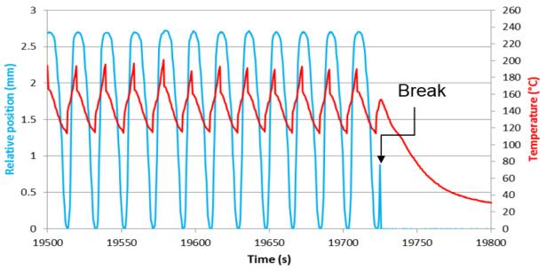
Figure 12. Cycles 7646-7657, load 70 MPa, stroke 2.7 mm, current 1.94 A
