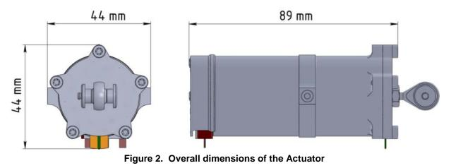
The overall dimensions of the developed actuator are shown in Figure 2.
