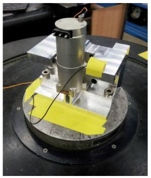
Figure 16. Axial vibration of the Actuator
