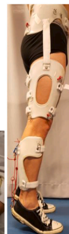
Fig. 1. the exoskeleton "MIKE" (Muscle contracture Induced by an Exoskeleton) with example of emulate contracture at the gastrocnemius and soleus muscles with visualization during standing before walking.
