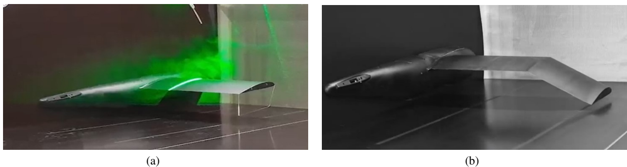
Figure 5: Semi-span setup, with PIV plane at about 26% wing-length from the root. Various wing tips were used, among which (a) a vertical plate, and (b) an anhedral section (keeping the vertically projected wing area constant).
