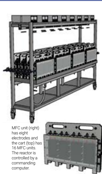
The team has upscaled previous work to create a 1,000-litre microbial fuel cell under a wastewater treatment plant in Sion, Switzerland.
