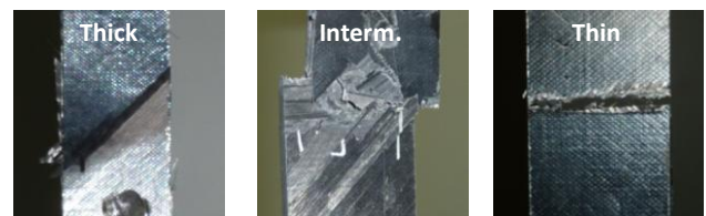
Fig. 4: Failure modes observed in quasi-isotropic uniaxial tensile tests: transverse cracking and delamination failure for thick ( n=1 ), multimode failure for intermediate ( n=3 ) and fiber dominated failure for thin ply laminates ( n=10 )
