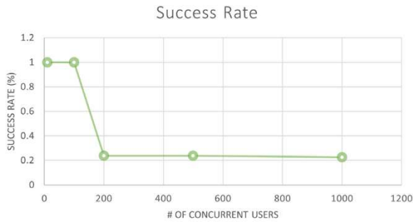
Fig. 8. Percentage of requests that are successful plotted against the number of concurrent users.
