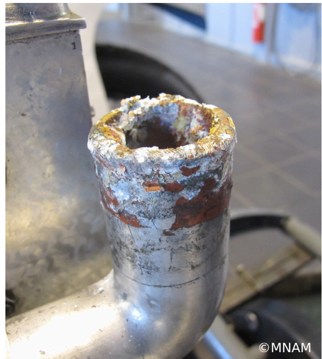
Figure 3. Metal heavily corroded under the hose of a Bugatti T28
