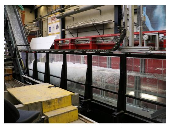
**Figure 2.** Photo of the spillway model with  $Q = 0.14 \text{ m}^3/\text{s}$ , the 50° smooth chute in the background and the plain stilling basin at the front. Flow direction from left to right.
