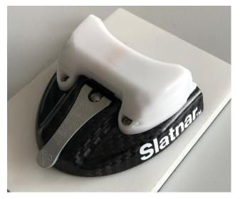
**Figure 2.** Attachment of the wearable tracker on top of the binding of the skis. The tracker is mounted on top of the regular ski jumping binding in front of the foot (tracker in white).
