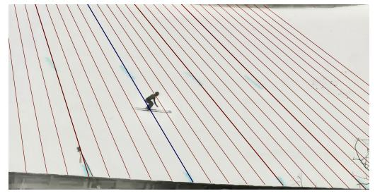
**Figure 3.** Example for the manual determination of the official video-based jumping distance. The red lines are the calibrated projection of the official jumping distance (to the jump-off platform). The blue line corresponds to the determined jumping distance.
