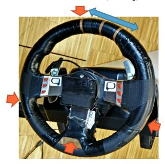
Figure 2. Logitech G27 Steering Wheel equipped with capacitive sensors, also called WheelSense. Red arrows depict hand-taps and blue arrow the hand-swipe.
