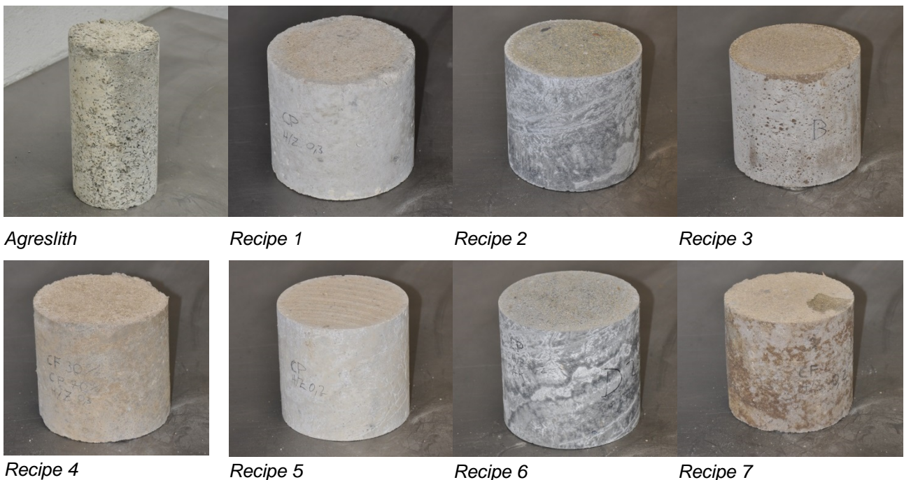
Figure 1 Visual aspects of hardened WCC specimens from different recipes.
