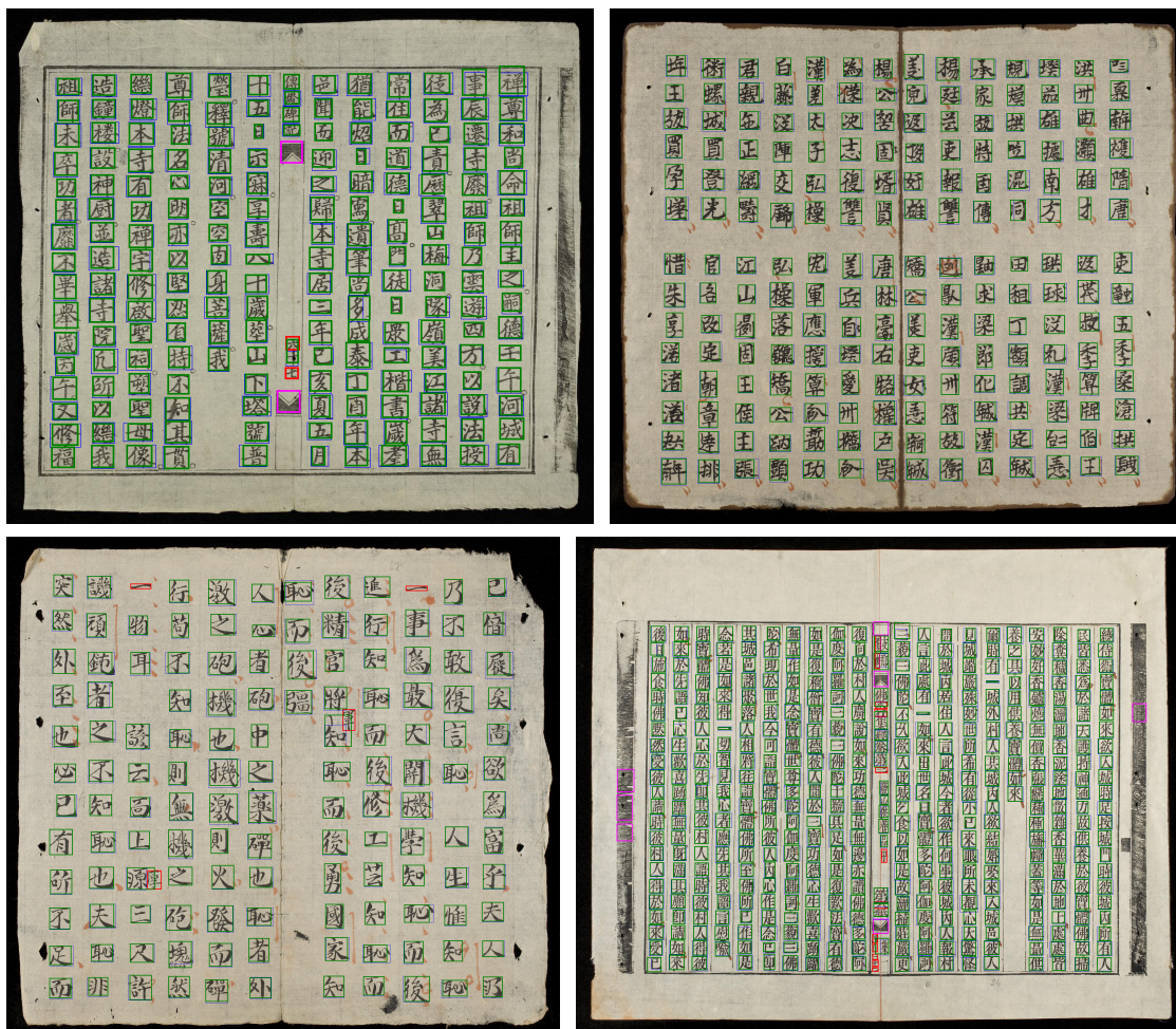
(c) Adapted character detection with YOLOv5m. Matching bounding boxes \mathcal{M} are green, insertions \mathcal{I} are magenta, deletions \mathcal{D} are red, and the ground truth is blue
