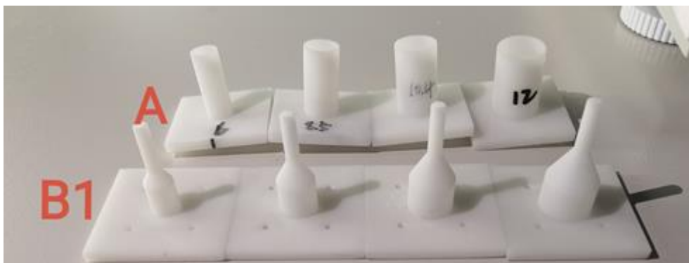
Figure SM10. Device architecture and mesh holder. A schematic representing the assembly of the mesh in the holder (top) and different mesh holders used to evaluate the flow rate independence are shown (bottom).
