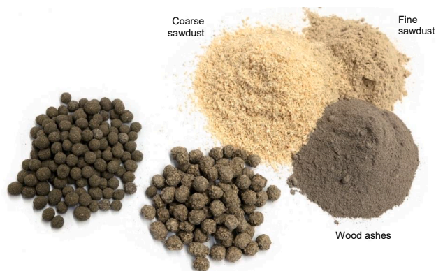
Fig. 1. Main raw materials (besides Portland cement) and two examples of pellets obtained from different raw material mixture formulations.
