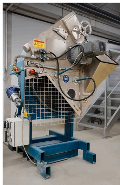
Fig. 3. Rotating drum pelletizer used in the reported study.
