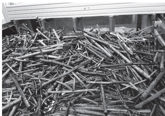
Figure 4. Photo of the driftwood blocked at the model weir, for the set-up without countermeasures ( \chi_R=1 , b/L_M=0.77 , V).
