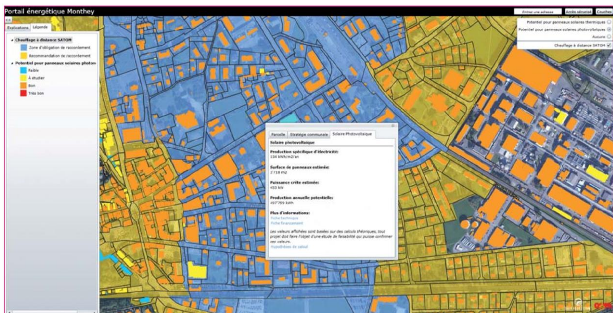
Figure 6 : Online map of solar photovoltaic cadaster and DHN deployment areas; Pop-up windows give specific building and land parcel information concerning solar energy potential and recommended heating technologies
