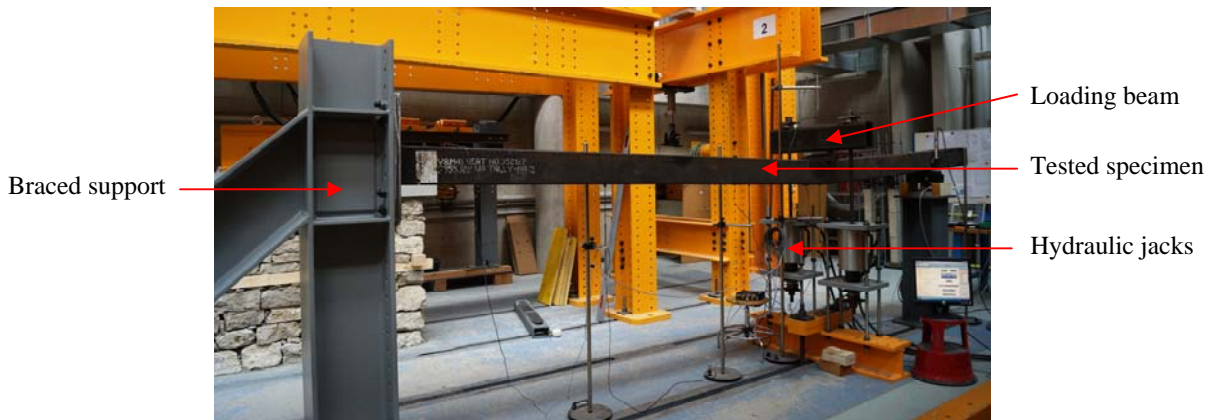
Figure 19: Deflected shape of a propped cantilever off-centrally loaded
