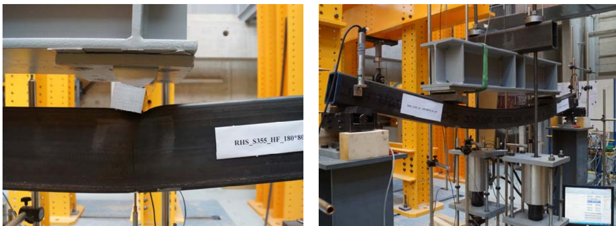
Figure 13: a) Onset of local buckling for RHS_180x80x4.5 – b) Deflected shape of RHS_150*100*8
