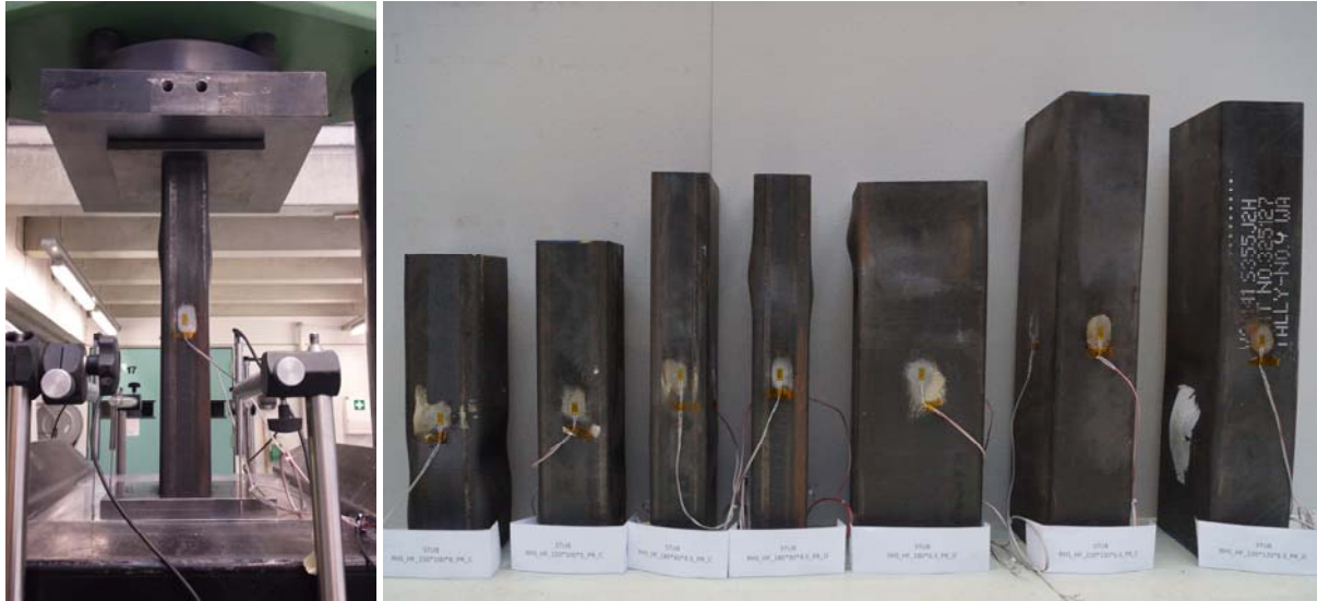
Figure 4: General test set-up and failure shapes of stub columns
