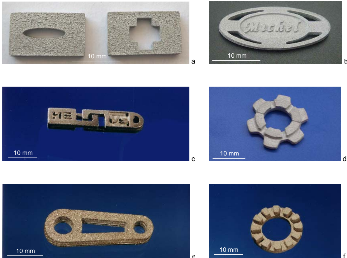
Figure 5: Finished parts on 17-4PH stainless steel (a, b, c, e), 316L stainless steel (d) and FeNi alloy (f)
