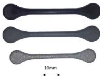
Figure 1: green, brown and sintered Ti6Al4V parts
