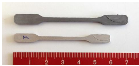
Figure 4: PIM P558 austenitic steel green (top) and sintered (bottom) specimens.
