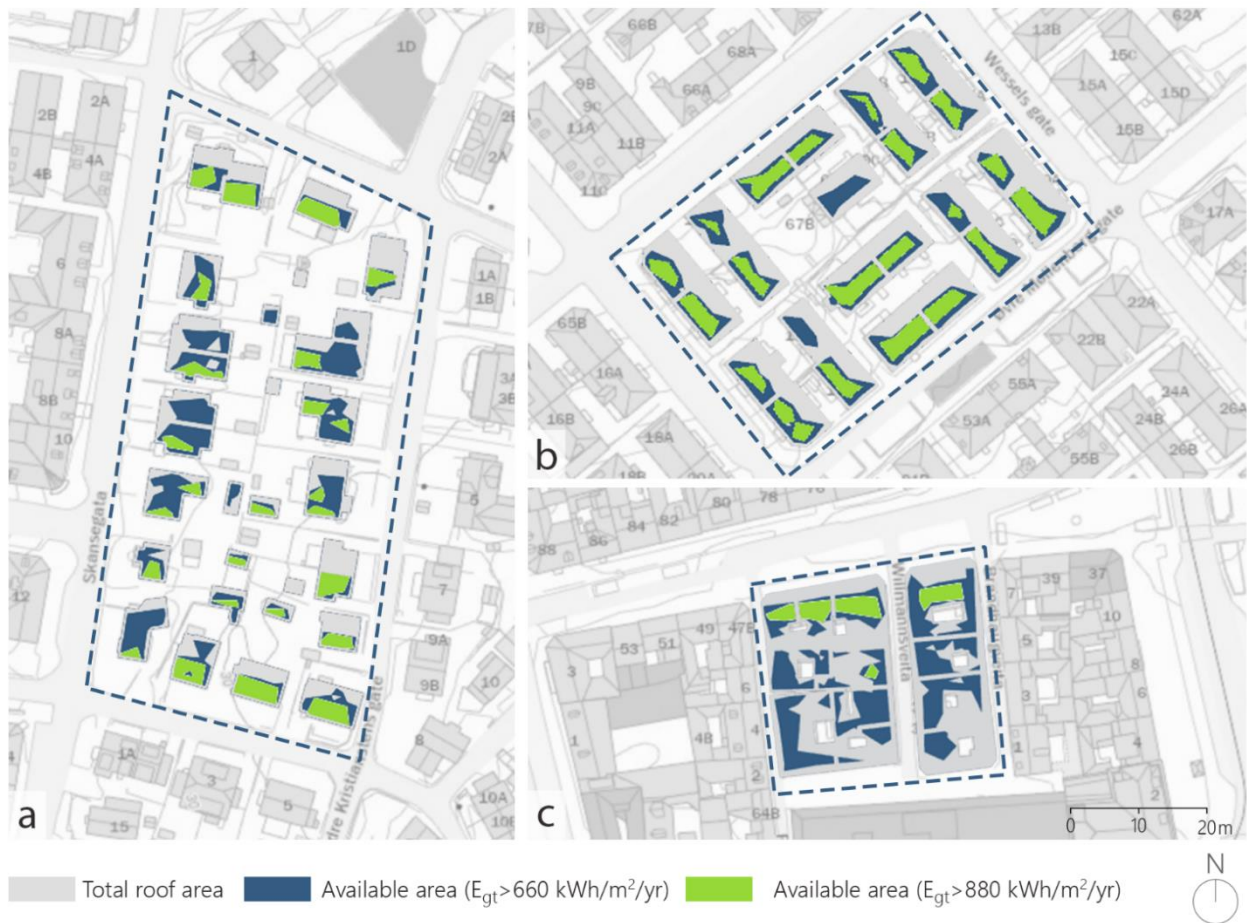
Figure 4: Available roof area resulted considering E_{gt} higher than 660 kWh/m 2 /yr and 880 kWh/m 2 /yr.
