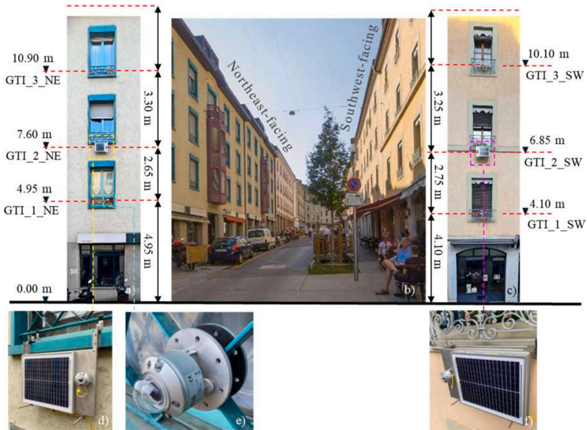
Fig. 2. Monitoring in the urban canyon Rue des Grottes: pyranometer placements on the a) northeast-facing facade and c) southwest-facing facade; b) street view of the urban canyon; d) and f) autonomous solar power supply, battery and data logger Campbel Scientific CR1000 (R), fixed to the railing; and e) pyranometer.
