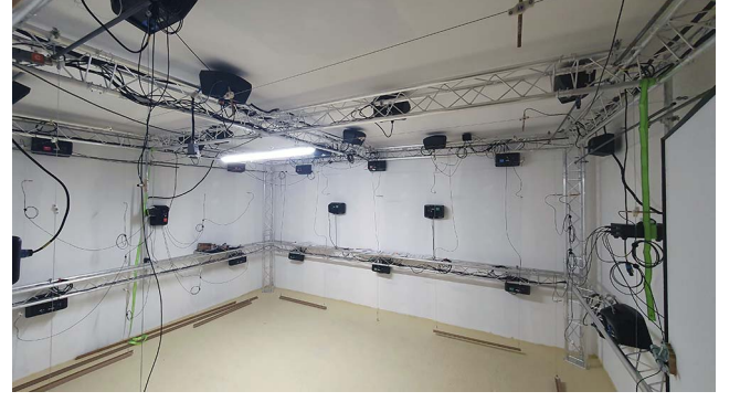
Figure 1. The LMA active set-up for controlling low-frequency wall reflections.
